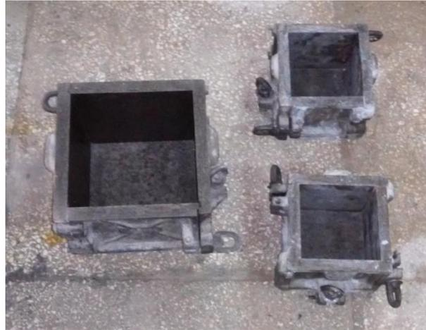
Figura 2.9: Moldes cúbicos de 100x100x100 mm y 150x150x150 mm
