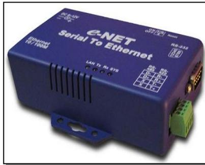
**Figura 2. 1: Convertidor e-NET Serial To Ethernet.**
