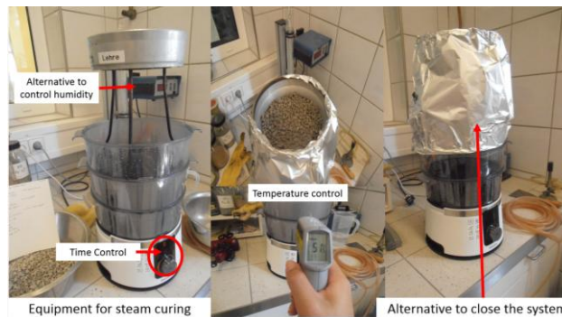
Figure 2 : Steam curing system
