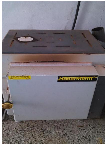
**Figura 2.11** Mufla Nabertherm.
