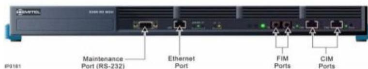
*Figura 2.1: Panel frontal del NSU (Network Service Unit)*
