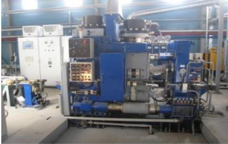
**Figura 2.1. Máquina de soldar carriles MCP- 6301A TB3.**
