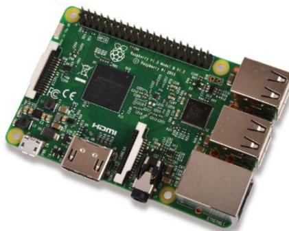
Figura 2.4 Raspberry Pi 3 Modelo B.
