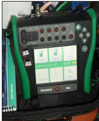
**Figura B-4.2:** Calibrador de campo y comunicador BEAMEX-MC6
