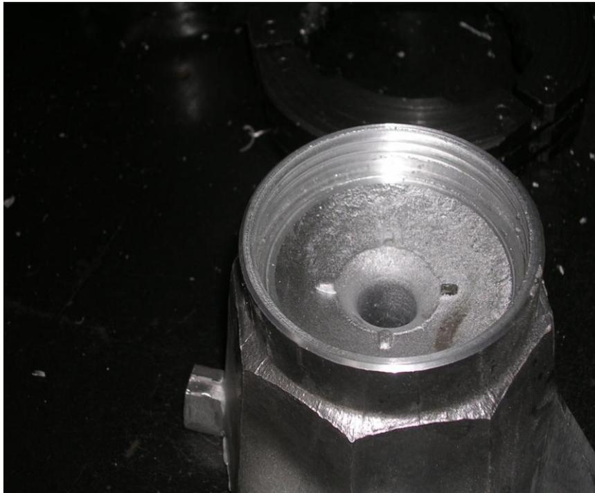
**Anexo VII. Vaso inferior colocado en la mordaza.**
