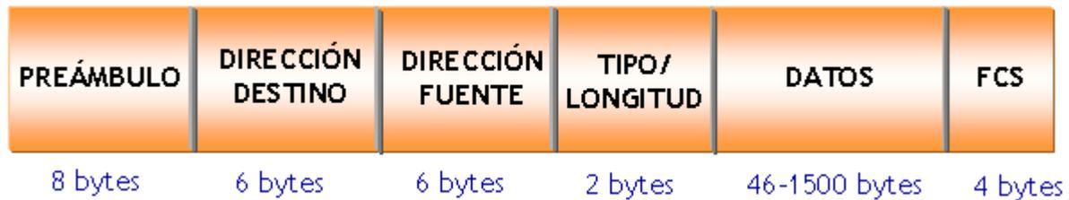
**Figura 5:** Protocolo Ethernet / 802.3.
