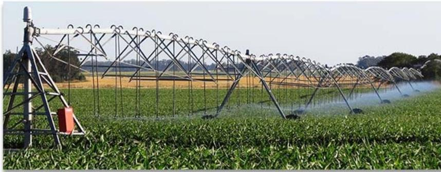
Figura 1. Máquina de Riego de Pivote Central (Valley Irrigation, 2017).
