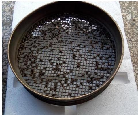
Figura 2.3. Tamiz No.4. Norma ASTM c-3 147/92.
